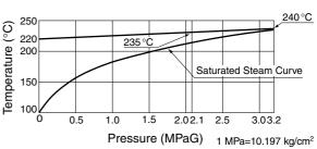
PRESSURE SHELL DESIGN CONDITIONS (**NOT** OPERATING CONDITIONS): Maximum Allowable Pressure (MPaG) PMA: 3.2 Maximum Allowable Temperature (°C) TMA: 300
