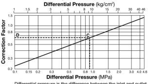
Differential pressure is the difference between the inlet and outlet pressure of the trap.
